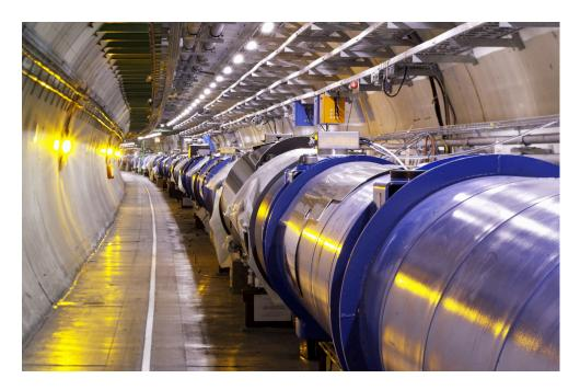
Figure 14: The LHC dipole magnets.
